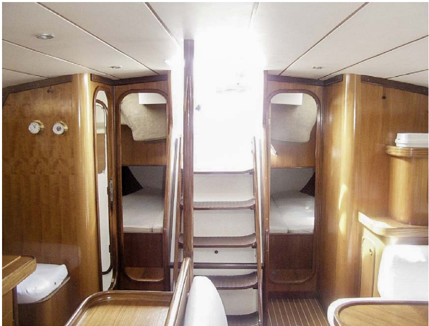
Fig. 13 High-quality lightweight panels finished in traditional high-gloss wood veneer and bonded using Sikaflex®-292i
